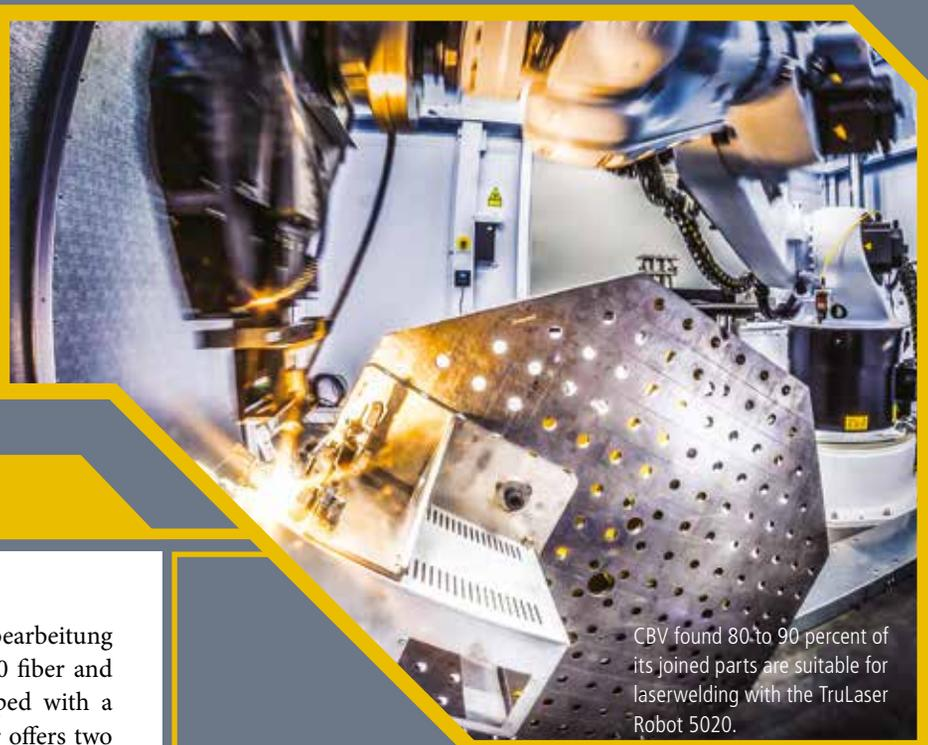
CBV found 80 to 90 percent of its joined parts are suitable for laserwelding with the TruLaser Robot 5020.
