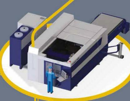
Here, the TruLaser 3030 fiber shares its TruDisk laser with the TruLaser Robot 5020, exhibiting the unique flexibility of the TruDisk laser resonator design.
